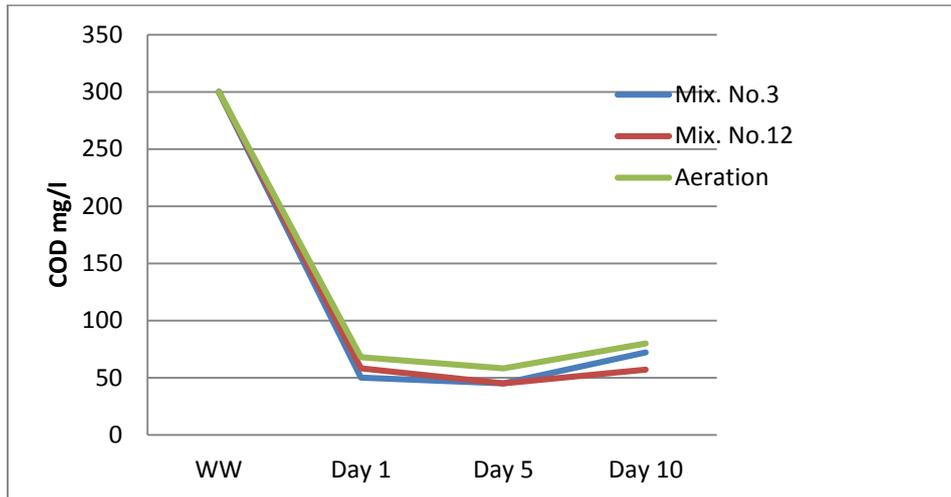
Fig. (3) Removal efficiency of COD in days.
