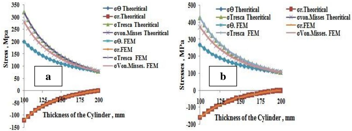
Figure 2 : Validation of analytical and FE simulation results at different operating pressure;
