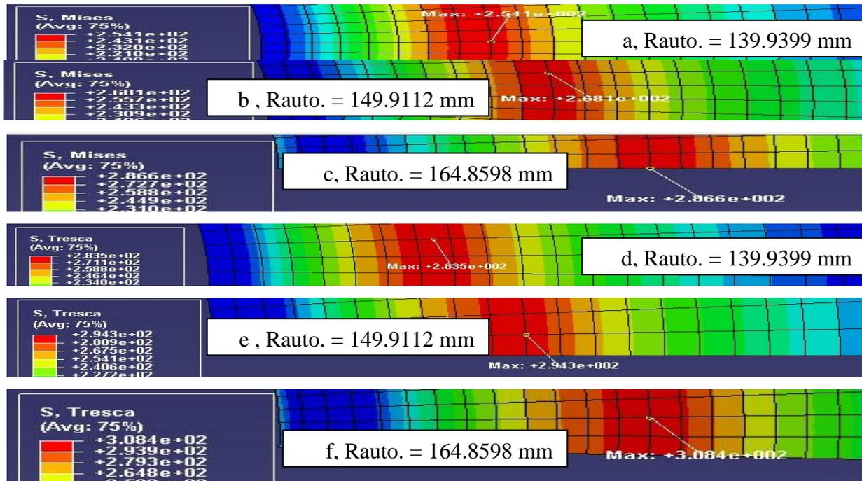
Figure (8) : FE simulation results of location of maximum *vonMises* ( a, b, c ) & *Tresca* ( d, e f ) stresses at operating pressure of ( Popr. = 140 MPa ) & different autofrettage pressure; a & d ) Pauto. = 320 Mpa , b & e ) Pauto. = 340 Mpa, c & f ) Pauto. = 360 Mpa .
