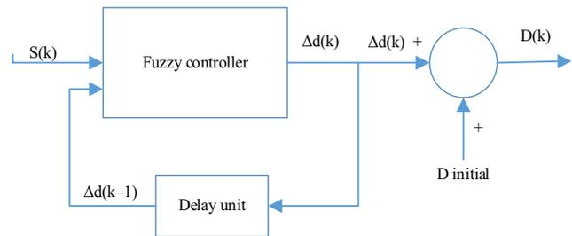
output is the new implied change of duty ratio (Δd). After the inputs are calculated and converted to linguistic variables, their universe of discourse is divided into five fuzzy subsets denoted as positive big (PB), positive small (PS), zero (z), negative small (NS) and negative big (NB). This implies that the proposed FLC has 25 rules as depicted in Table II, while Figure 6 below reveals the membership functions for the FLC's input and output, respectively.
