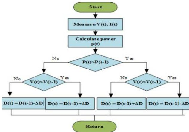
convergence toward the MPP and higher efficiency than a conventional one (Femia et al., 2004). However, the modified type also malfunctions during rapid environmental changes.
